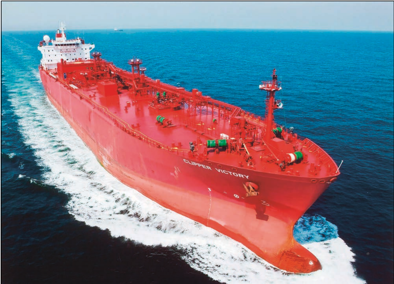
Figure 5.1 The Norwegian fleet is modern and specialised in technologically advanced, capital-intensive segments. Pictured is an LPG tanker, designed for transporting liquefied petroleum gas.
