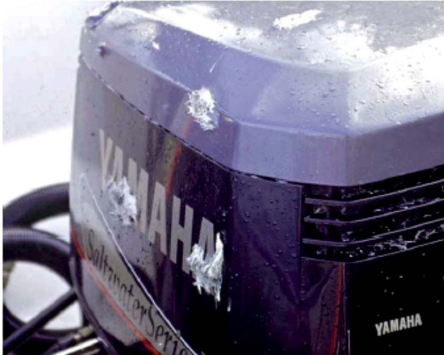
When 'stop' really does mean 'stop'; a tight group of disabling shots shot-out these go-fast boat engines fired by a marksman from a MH90 Enforcer helicopter during a cocaine bust off the coast of Florida.
