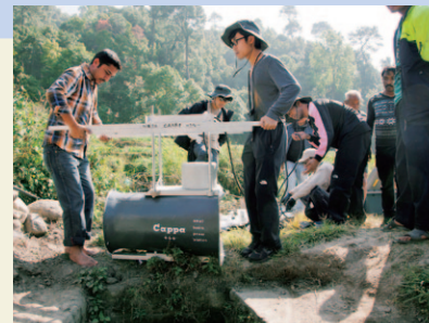
The small hydro-kinetic power generator “Cappa” which can be carried by two adults by hand (Photo: ibasei)
