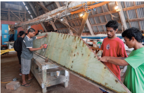
A vocational training center located on the Majuro Atoll in Marshall. Students build an outrigger canoe using traditional techniques inside a facility constructed through the Grant Assistance for Grass-Roots Human Security Project. (Photo: Hideyuki Yamasaki / Embassy of Japan in Marshall)
